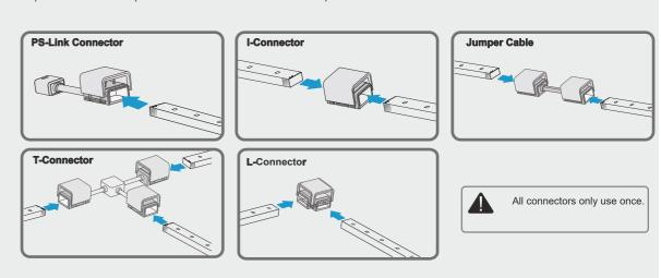
**B** Push the strip completely into the connector.
