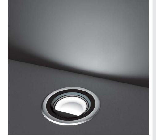
Diameter 205mm ground-recessed luminaire for outdoor installation, phosphochromatised and polyester powder coated die-cast copper-free aluminium body and stainless steel AISI 316L frame, tempered safety glass, moulded silicone gasket. Built-in LED driver 220-240V 50-60Hz, , with 32 x mid-power SAMSUNG 2835 LED. IP67 rating.
