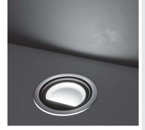
Diameter 240mm ground-recessed luminaire for outdoor installation, phosphochromatised and polyester powder coated die-cast copper-free aluminium body and stainless steel AISI 316L frame, tempered safety glass, moulded silicone gasket. Built-in LED driver 220-240V 50-60Hz, , with 66 x mid-power SAMSUNG 2835 LED. IP67 rating.
