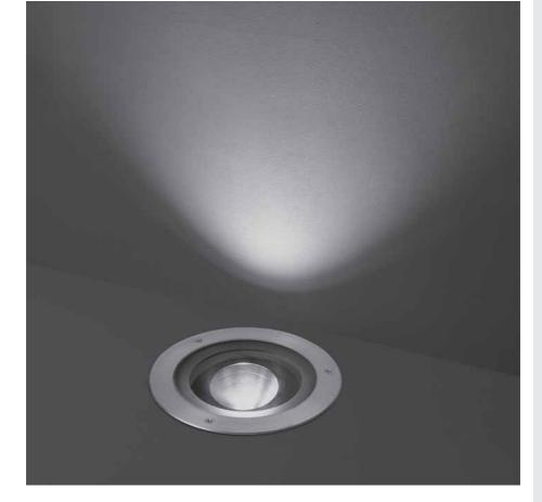
Ground-recessed luminaire in round shape for outdoor installation, phospho-chromatised and polyester powder coated die-cast copper-free aluminium body and stainless steel AISI 304 frame, tempered safety glass, moulded silicone gasket. Symmetrical light distribution with adjustable optics. Built-in LED driver 220-240V 50-60Hz, with 1 CREE CXB 3050 COB LED. IP67 rating.
