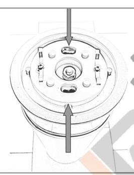
7— insert the luminaire in the cylinder and pay attention to the correct symmetrical position of head cup fixing holes (must be perpendicural to the light beam direction) fix it by screwing the nut
