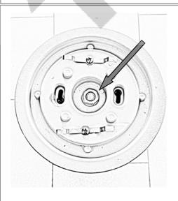
2– remove the fixing nut by unscrewing it
